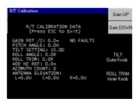
FSD outer knob to perform tilt adjustments, the inner knob to perform roll trim adjustments, and the Gain UP and Gain DOWN soft keys to make gain adjustments.
