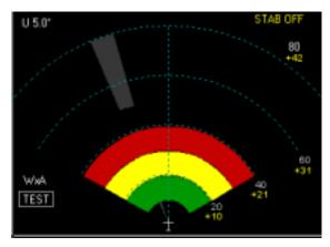
FIGURE 40: Typical Test Pattern
