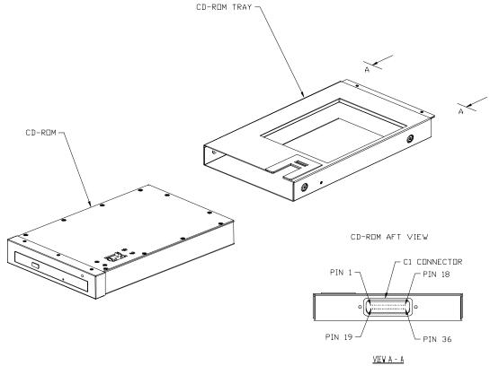
FIGURE 2: CD Data Loader Exploded View
