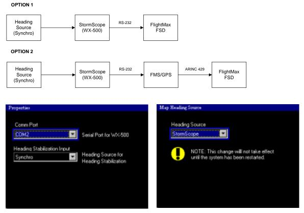
FIGURE 15: Lightning Properties and the Map Heading Source
