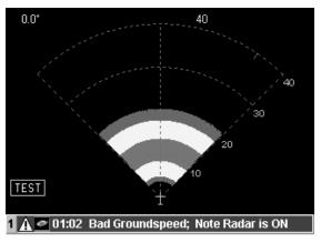
FIGURE 37: Typical Test Pattern Display
