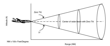
FIGURE 32: Radar Beam Illumination
