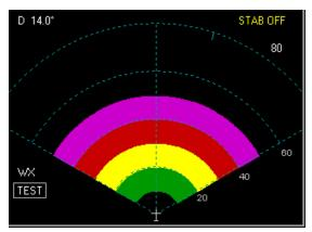
FIGURE 52: Typical Test Pattern Display
