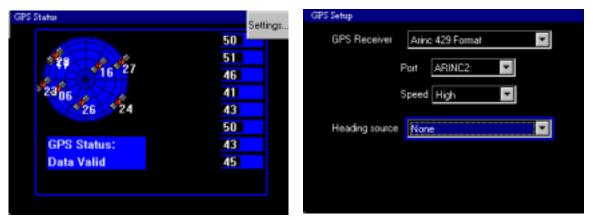
FIGURE 12: GPS Status and Setup Pages (ARINC 429)
