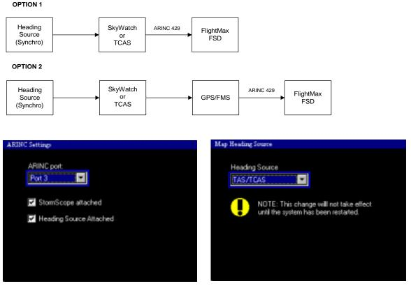
FIGURE 16: ARINC Settings and the Map Heading Source
