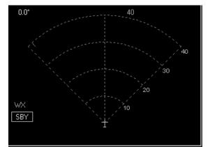
Adjust the tilt control to -5, -10, -15 checking that the antenna tilts smoothly and without interference. For a DA-144A array antenna, -15
