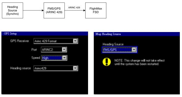
FIGURE 14: GPS Setup Page and the Map Heading Source Page
