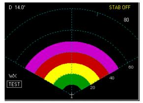
FIGURE 55: Typical Test Pattern Display
